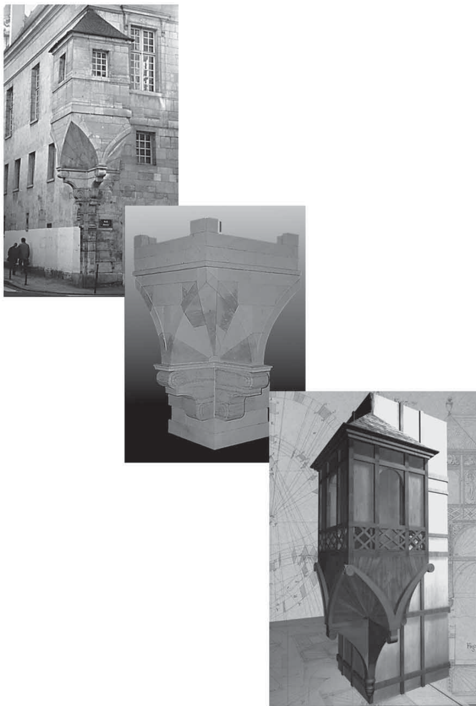
Figura 4. Composizione di trompes coniche in rue des Francs Bourgeois (Parigi): modello lapideo e ligneo secondo Emy. Composition of conic trompes in rue des Francs Bourgeois (Paris): stone and wood model according to Emy.
